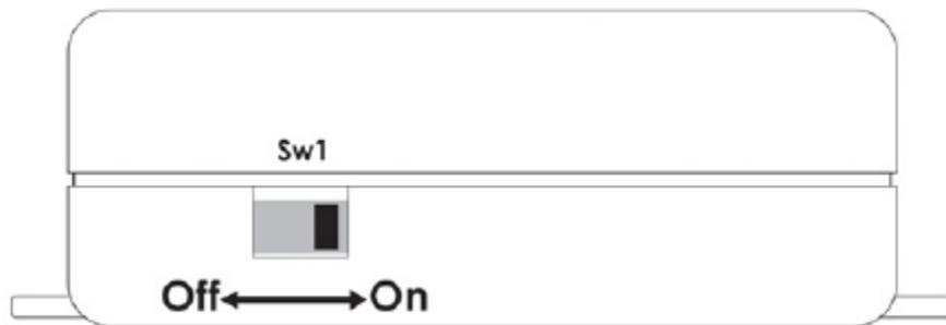
Now Carman is equipped with the supporting battery, and this battery provides electrical power of the device when the car's main power is disconnected. You will be informed by SMS if car's main power is disconnected. Carman system can work with supporting battery for about 8 hours if it keeps sending information every 5 minutes. Note that if car's main battery gets disconnected, anti-theft system will not be working and only car tracing item will work.
